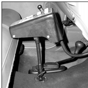
Adjustable Pedestal Mount (For use with all controls) P/N 63078 (12" Shaft)
