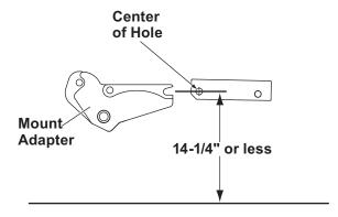
If measured height is 14-1/4" or less, no height adjustment is needed.
