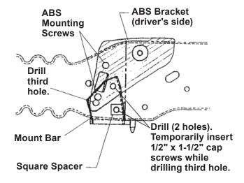
3. Use the formed plates as templates for drilling four 9/16" holes in each side of the vehicle frame. (Only three holes need to be drilled if the vehicle has a pre-existing slot.) Install two nut bars to the inside of each vehicle frame rail, aligning them with the drilled holes.
