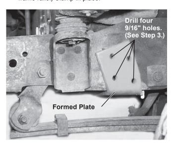
NOTE: Vehicles with an ABS bracket, as shown in diagram, require the following additional steps A through F to install the formed plate on driver's side.
