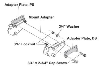
Repeat for the passenger's side. Tighten all fasteners according to the torque chart.
