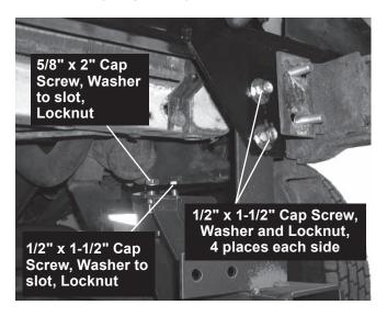
10. Loosely attach the cross bar between both mounts using 1/2" x 1-1/2" cap screws and locknuts.
