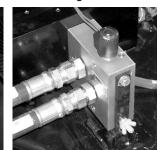
11. Get the response you demand from your plow with this easy-to install add-on and experience increased power and speed to all of the plow hydraulic functions! The auxiliary manifold bolts right up to the existing manifold and pump bracket without any modifications needed. Manifold provides up to 30 gpm input (4000 psi max.) from the vehicle pump and 2-3 gpm output (2500 psi max.).
