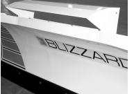
**5.** Help channel air flow to your truck radiator during the long haul over the road. Mounted front and center, our custom airfoil redirects air over the top of the blade and into the grill of your vehicle. The airfoil is shipped with complete mounting hardware.
