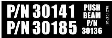
A label identifying the undercarriage assembly part number and push beam part number is applied to the rear of the push beam.
