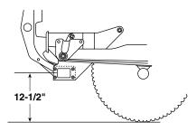
The recommended push beam height for this undercarriage assembly is 12-1/2" from the center of the push beam to level ground. DO NOT exceed 14-1/2" in height for this undercarriage.
