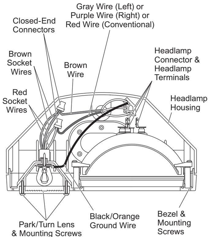
1. Remove two screws from park/turn lens and remove the lens.
