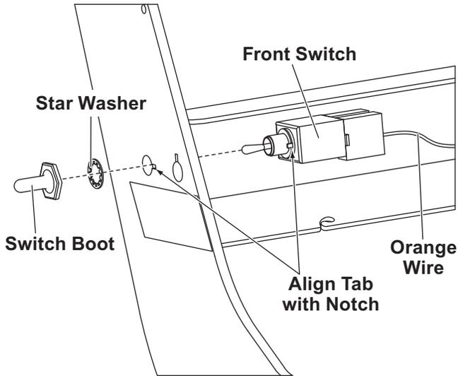
4. Tighten until the switch is firmly in place.
