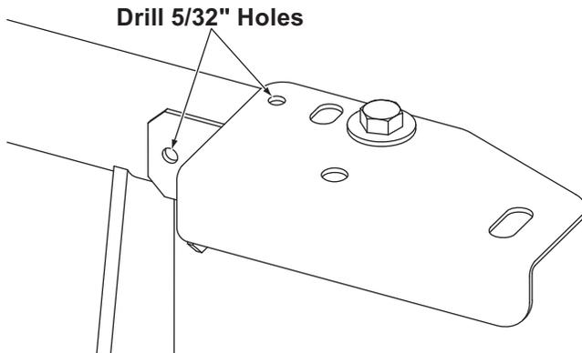
Insert a 1/4" x 3/4" self-tapping screw in each hole. Tighten all fasteners and mount the headlamps as described in the Mounting Headlamps to Extension Brackets section of these instructions.
