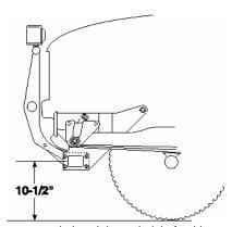
The recommended push beam height for this undercarriage assembly is 10-1/2" from the center of the push beam to level ground. DO NOT exceed 12-1/2" in height for this undercarriage.
