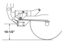
The recommended push beam height for this undercarriage assembly is 10-1/2" from the center of the push beam to level ground. DO NOT exceed 12-1/2" in height for this undercarriage.
