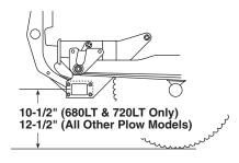
The recommended push beam height for the 680LT & 720LT undercarriage assembly is 10-1/2" from the center of the push beam to level ground.
