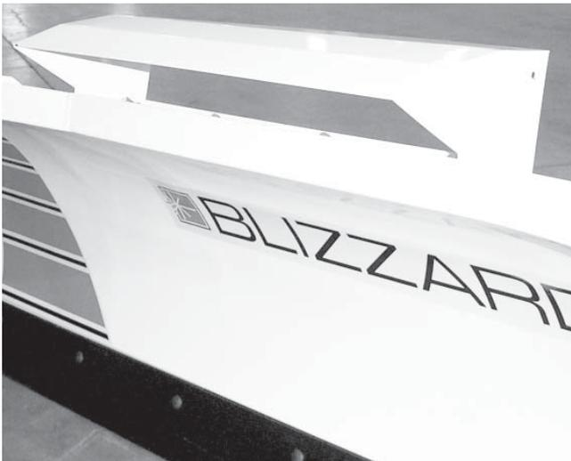
5. The snowplow airfoil helps channel air flow to your truck radiator during the long haul over the road. Mounted front and center, our custom airfoil redirects air over the top of the blade and into the grille of your vehicle. The airfoil is shipped with complete mounting hardware.
