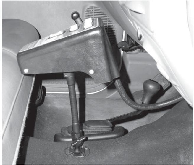
6. Our easy-to-install, adjustable pedestal mount kit will position either POWER PLOW™ snowplow control station how you want it! Ideal for bucket seat vehicles with low center consoles. Pedestal accessory shipped with complete hardware and adapter plate.
