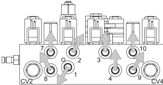
**NOTE:** The arrows shown on the manifold illustration indicate the direction the 90° adapters should be positioned to receive the hydraulic hoses.
