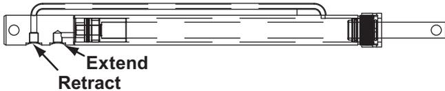
**NOTE: The hoses that operate the retract functions (rod) of the cylinders are closest to the base of each cylinder. The hoses that operate the extend functions (base) of the cylinders are closest to the rod of each cylinder.**
