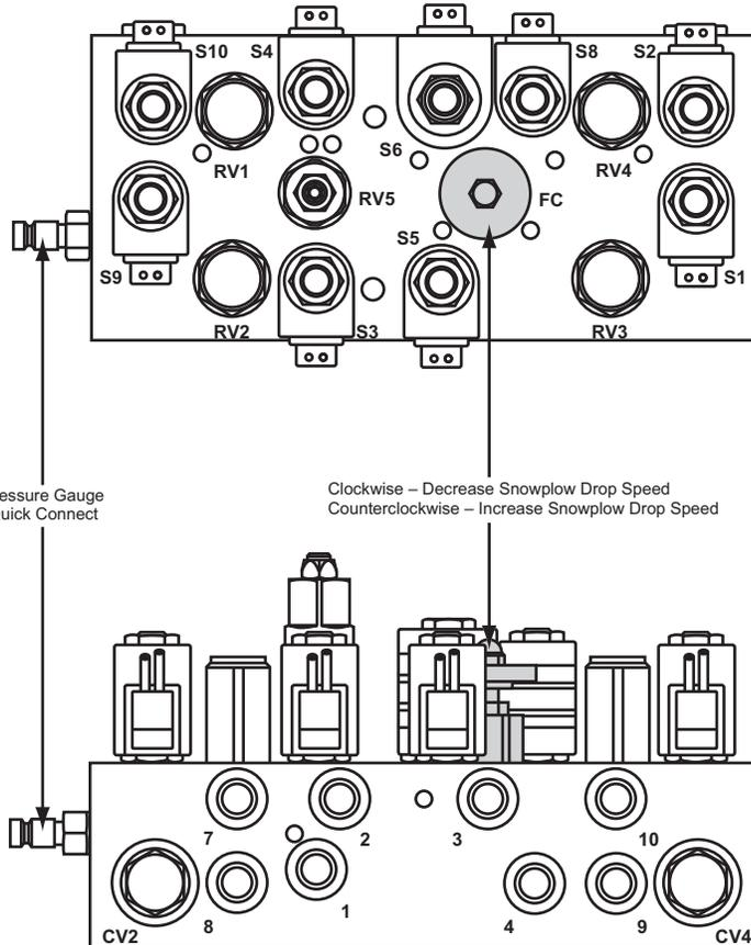
NOTE: Check valves CV1 & CV3 are not illustrated. Both valves are located on the opposite side of the manifold in the diagram shown above.
