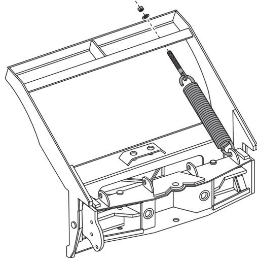
15. Install the blade guides at each end of the moldboard. Insert the cap screw through the holes at the top of the wing reinforcement rib. Tighten all screws with locknuts.
