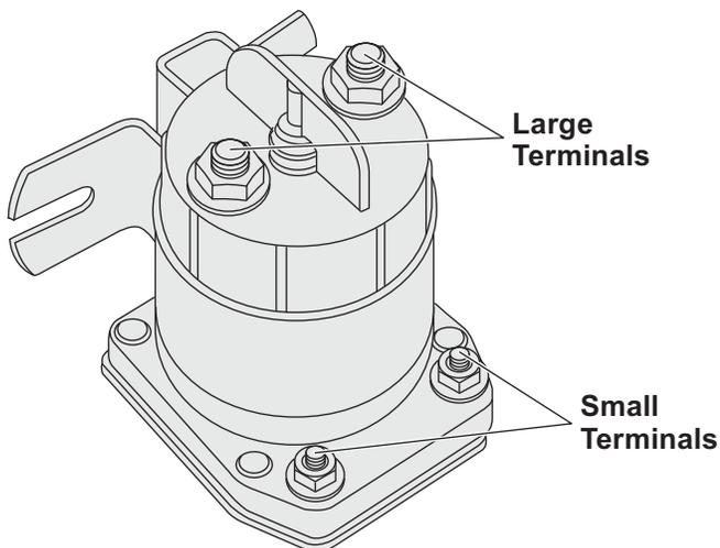
the eyelet terminal onto it. Attach the eyelet to the remaining small terminal on the contactor. Secure it with the hardware provided on the solenoid.
