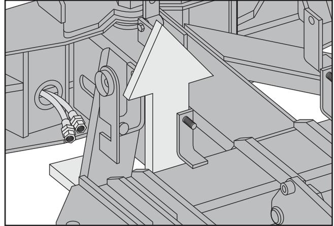
Feed each group of hoses (two per side) through the grommets in the pivot beam and up through the openings in the A-frame. Positioning the hoses through the pivot beam supports the hoses while the snowplow is in use and prevents them from dragging on the ground.
