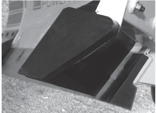
8. Durable and long lasting, the POWER PLOW™ polyurethane moldboard and wing cutting edges will keep you plowing longer and safer. Specially formulated for snow plowing applications, BLIZZARD® poly edges resist gouging, provide superior wear life, and effectively reduce plowing noise. Ideal for all plowing conditions. Edges are shipped with mounting hardware.
