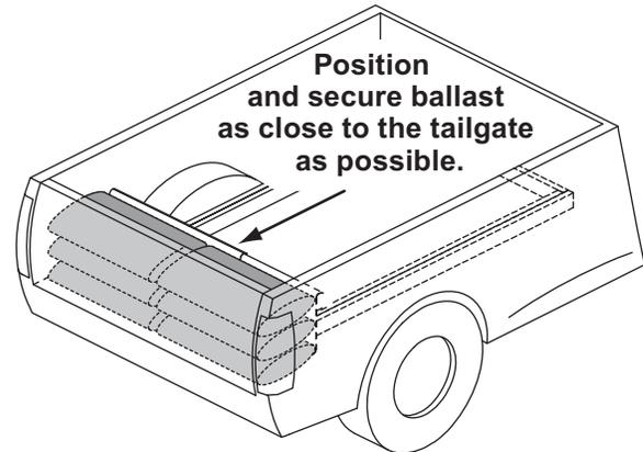
Ballast (additional weight) is an important part of qualifying vehicles for snowplow eligibility. Rear ballast must be used when necessary to remain in compliance with axle ratings and ratios as specified by the vehicle manufacturer.
