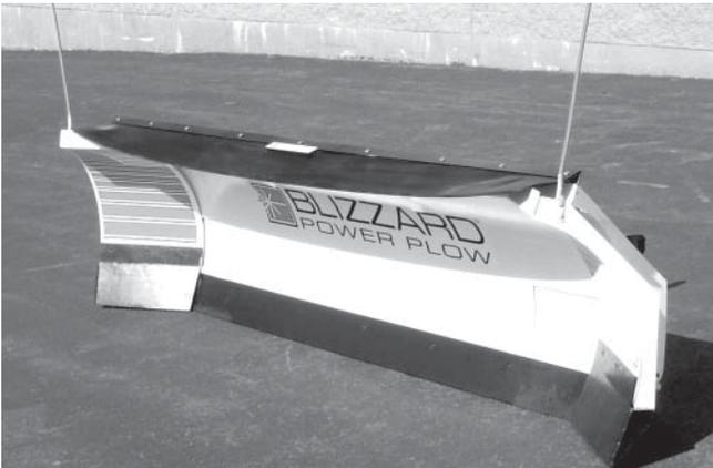
2. Rugged and durable, the 3/8" thick, 2-ply rubber snow deflector keeps snow off your windshield and in its place—on the ground! One-piece design allows for wing clearance and provides optimum snow deflection. The deflector is shipped with a POWER PLOW™ vinyl label and complete mounting hardware.
