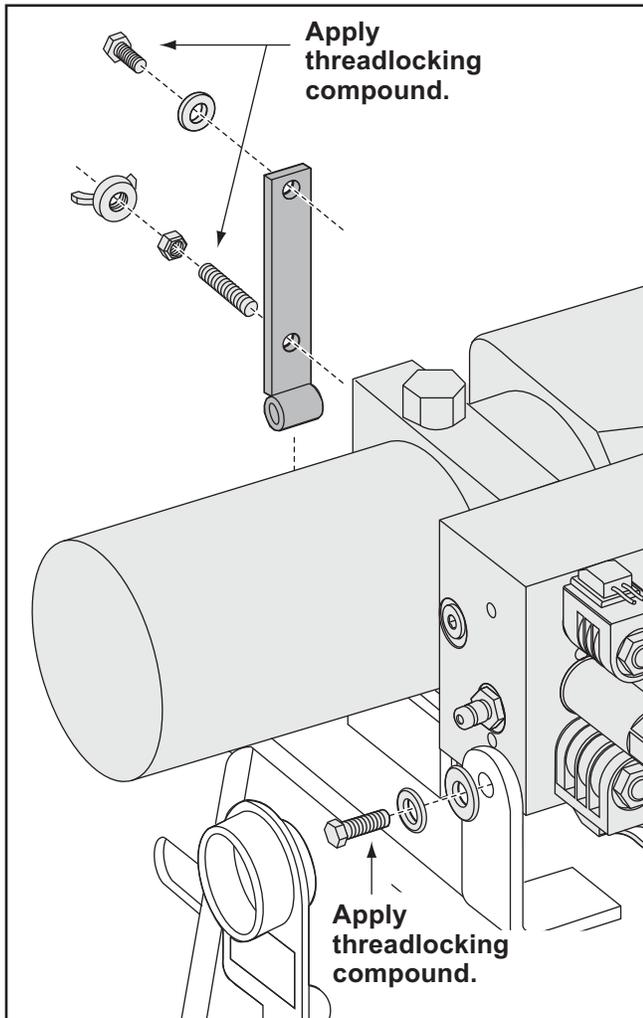
**NOTE: A medium-strength threadlocking compound should be used to secure the manifold mount fasteners.**
