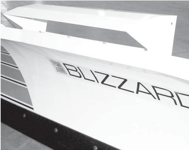
1. The snowplow airfoil helps channel air flow to your truck radiator during the long haul over the road. Mounted front and center, our custom airfoil redirects air over the top of the blade and into the grille of your vehicle. The airfoil is shipped with complete mounting hardware.
