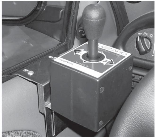
4. This adjustable bracket mounts easily to your straight blade joystick control and installs quickly onto any door panel. Ideal for left-hand joystick operation or for vehicles with center consoles. The window mount bracket is shipped complete with hardware. Some assembly required.
