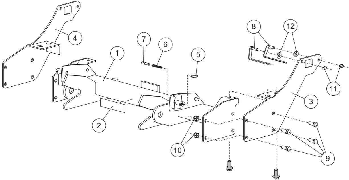
Shaded parts are original vehicle fasteners.
