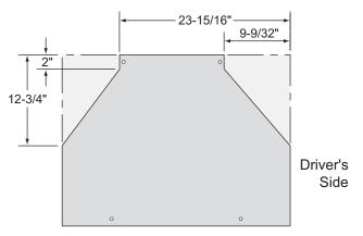
10. Position the splash shield on the vehicle so that the tapered end is toward the rear and the shield is on top of the mount and below the vehicle sway bar.
