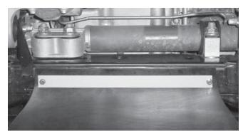
12. Make sure the splash shield is under the vehicle sway bar, then pull the uncut end of the shield to the vehicle bumper support beam.
