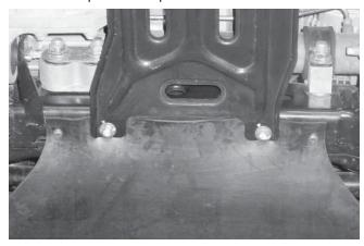
If the vehicle is not equipped with a transaxle skid plate, align the holes in the rear splash shield retainer and the tapered end of the splash shield with those in the vehicle frame cross member. Install two M6 x 1.00 cap screws (supplied with the mount) through the rear splash shield retainer and splash shield and into the cross member. Do not overtighten.
