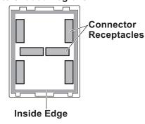
2. The plugs and switches are keyed to fit in the correct orientation. Ensure the body of the switch matches the plug before installing.
