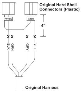
2. Remove 3/8" of insulation from the ends of the cut harness wires.
