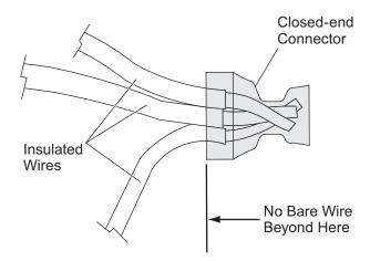
14. Verify that no bare copper wire is exposed beyond the opening of the closed end connector.
