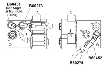
NOTE: Both lift cylinder hoses should be routed through the triangular openings in the A-frame. Position these hoses over the A-frame angle and to their respective manifold ports.
