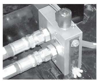
4. Experience increased power and speed in all of the snowplow hydraulic functions with this easy-to-install add-on central hydraulic valve block! The auxiliary manifold bolts right up to the existing manifold and pump bracket without any modifications needed. Manifold provides up to 30 gal/min input (4000 psi max.) from the vehicle pump and 2–3 gal/min output (2500 psi max.) to the existing hydraulic manifold. Hydraulic hoses, fittings, and pump not included.
