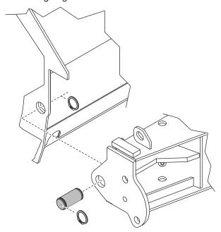
3. Mount the kickstand to the end of the pivot beam (driver's side) using the 1/2" x 4-1/2" cap screw provided. The spring, bushing and locknut are located on the inside of the pivot beam. Review the diagrams below and to the right. To pivot the kickstand, pull the spring-loaded leg out and rotate it until the pin locks into place. Adjust the foot on the stand arm so that the foot is 1/8" from the
