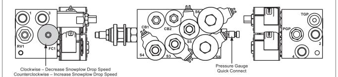
If being used with auxiliary hydraulics, recommended for systems having a flow rated at 4–30 gallons per minute (gpm) and a maximum pressure rating of 3,000 psi.
