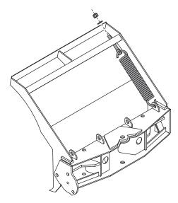
14. Install the blade guides at each end of the moldboard. Insert the cap screw through the holes at the top of the wing reinforcement rib. Tighten all screws with locknuts.
