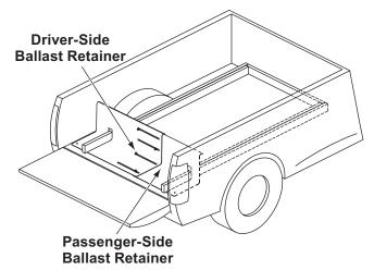
7. Ballast (additional weight) is an important part of qualifying vehicles for snowplow eligibility. Rear ballast must be used when necessary to remain in compliance with axle ratings and ratios as specified by the vehicle manufacturer. If ballast is required, it is important that it be secured properly behind the rear axle. A ballast retainer kit is available from your BLIZZARD outlet, PN 62849.
