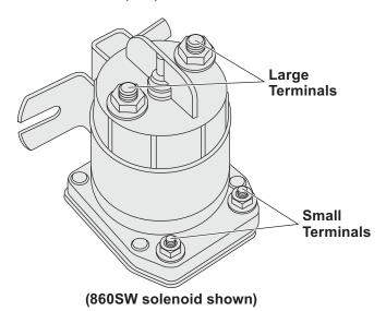
to length. Strip the end of the harness and crimp the eyelet terminal onto it. Attach the eyelet to the remaining small terminal on the contactor. Secure it with the hardware provided on the solenoid.
