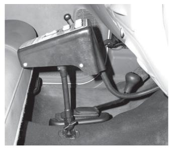
Our easy-to-install, adjustable pedestal mount kit will position either POWER PLOW<sup>™</sup> snowplow control station how you want it! Ideal for bucket seat vehicles with low center consoles. Pedestal accessory shipped with complete hardware and adapter plate.
