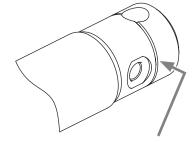
Current rams have a groove all around the base, near the pin hole. Early rams do not have a groove.
