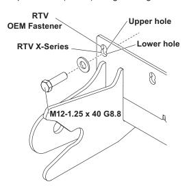
**For RTV X-Series Models:** Align the *lower* holes in the pushbeam with the holes in the bumper and frame, with the fasteners provided, See above. Reinstall the inner fasteners attaching the skid plate to the frame. Passing them through the rear arms of the pushbeam using shims provided. See following illustration.
