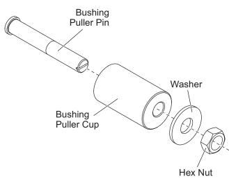
3. Insert the head of the puller pin into the bearing sleeve.
