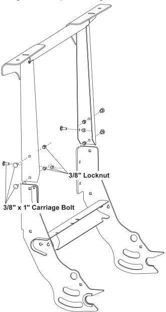
2. Secure with six 3/8" x 1" carriage bolts and locknuts assembled from the outside in.
