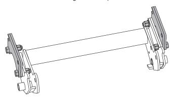
5. Position the mount adapter between the undercarriage brackets on each side. Align the notches in rear of the mount adapter with pins in
