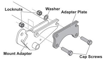
Repeat for the passenger's side. Tighten all four fasteners according to the torque chart.
