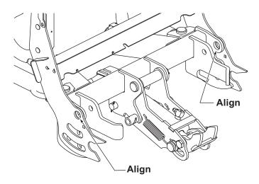
Insert the hitch pin cartridge through the hitch pin holes on the driver's side. Secure with a 3/8" x 1" carriage bolt and a 3/8" locknut assembled from the inside out. Repeat on the passenger's side.
