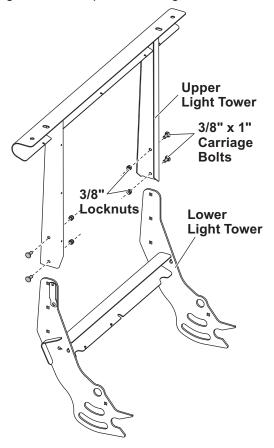
2. Secure with four 3/8" x 1" carriage bolts and locknuts assembled from the outside in.
