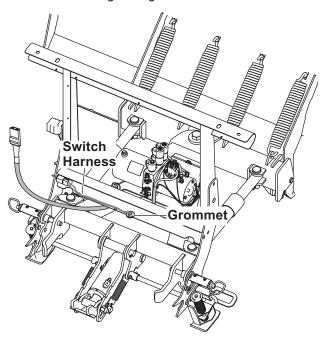
10. Bundle the remaining loose wires at the hydraulic unit with cable ties in the areas shown.
