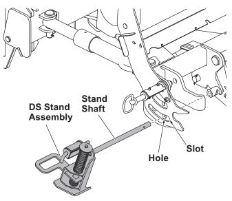
Lubricate the end of the shaft with general purpose petroleum grease. Guide the stand shaft into the draw latch bushing. Secure with 1/4" x 2-1/4" cap screw and 1/4" locknut. Do not fully tighten the 1/4" locknut. The cap screw must move freely through the slot in the draw latch bushing.
