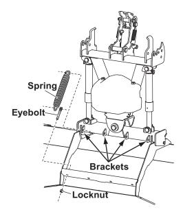
3. Push the threaded ends of the eyebolts through the holes in the spring bar on the blade. Attach a 5/8" locknut to each eyebolt.
