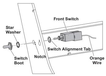
8. Repeat for the "Momentary ON, OFF, Momentary ON" switch in the hole farthest from the blade.
