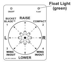
Moving the control lever in straight lines up and down or from side to side on the control body will result in the following blade movements:
