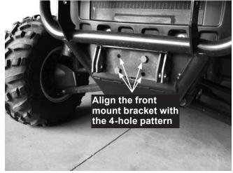
4. Slide the push assembly into the rear pins and rotate up to align front holes. Secure with supplied bent pins and hairpin cotters.
