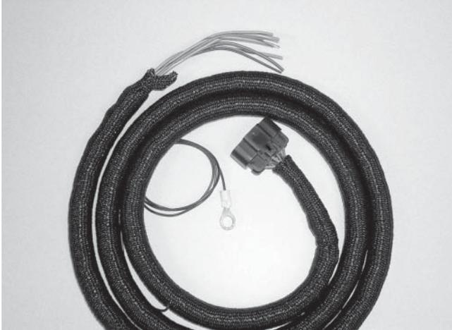
5. Integrate all snowplow controls into your skid steer using an optional auxiliary control harness. This 7-foot braided harness connects easily to your existing manifold harness on one end and your skid steer on the other. Assembly of the harness wiring to your skid steer-specific auxiliary electrical controls required. Electrical connector not provided with harness.
