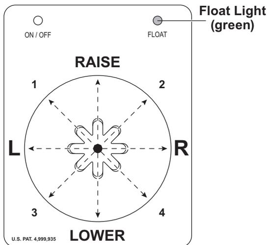
Moving the control lever in straight lines up and down or from side to side on the control body will result in the blade movements described in the following tables.
